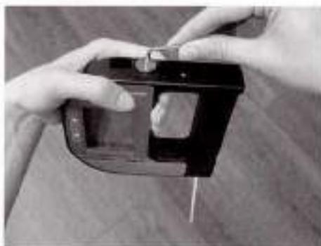
Fig. 11 - 3 Removing the battery cover
