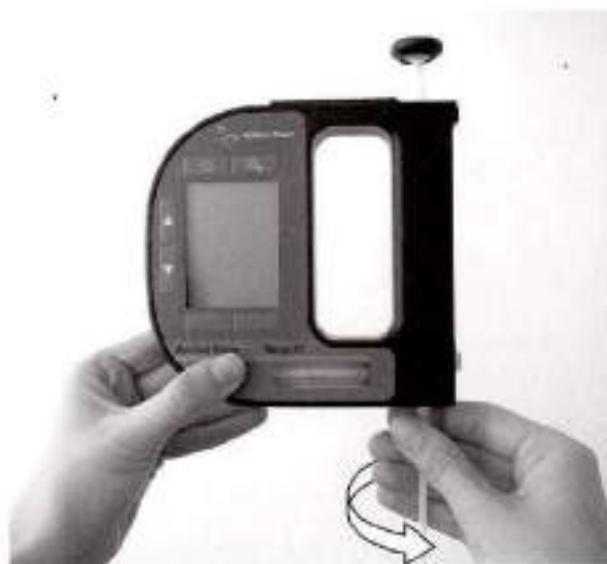
Fig. 7 - 1 Connecting the filling tube
