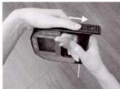
Fig. 11 - 2 Removing the pump lock
