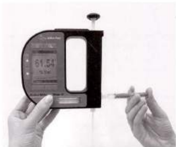
Fig. 9-3 Filling sample using the plastic syringe
