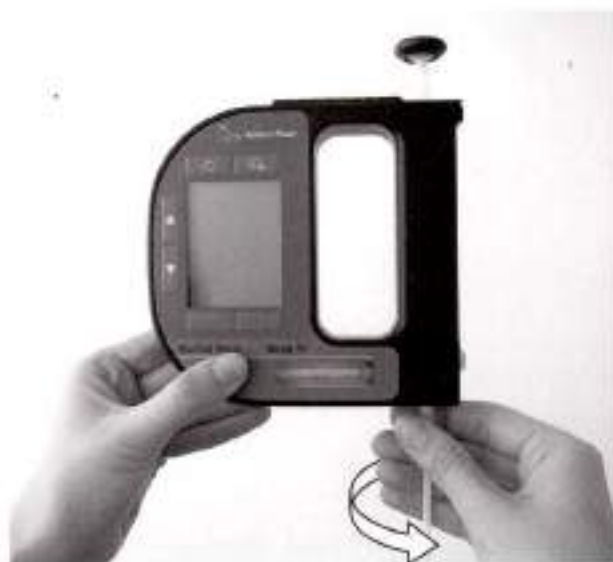
Fig. 7 - 1 Connecting the filling tube
