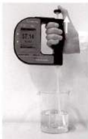
Fig. 9 - 2 Releasing the pump lever and reading the result
