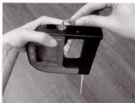
Fig. 11 - 3 Removing the battery cover
