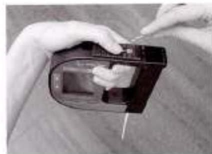
Fig. 11 - 2 Removing the pump lock
