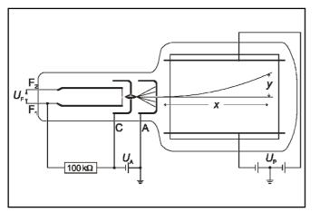
Fig. 2: Deflection in an electric field
