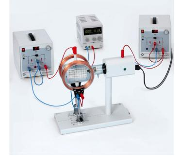
Fig. 1: Deflection in the electric field or in the magnetic field
