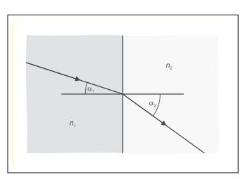
Fig. 1 Change of the direction of propagation at the interface between two media having different refractive indices
