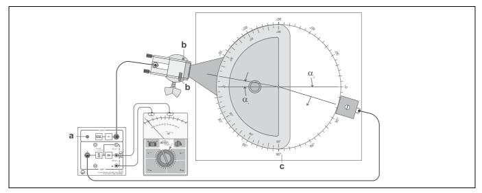
Fig. 3 Experimental setup for investigating the refraction of microwaves (view from above)
