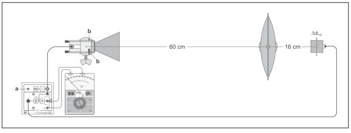
Fig. 4 Experimental setup for checking the focussing effect of a lens
