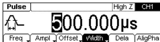
Figure 2-13 Pulse Signal Parameter Setting Interface
